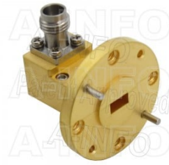
22WCA2.4_Cu Right Angle Rectangular Waveguide to Coaxial Adapter 33-50GHz WR22 to 2.4mm Female
