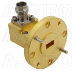
22WCAK_Cu Right Angle Rectangular Waveguide to Coaxial Adapter 33-40GHz WR22 to 2.92mm Female
